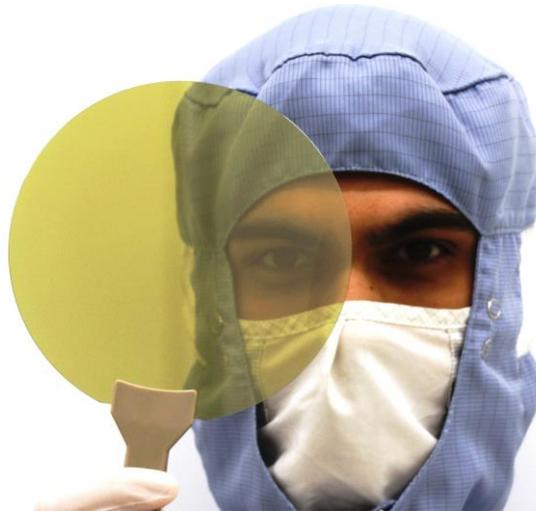
*Picture 1: 150 mm SiC epi wafer for high voltage power semiconductors.*
