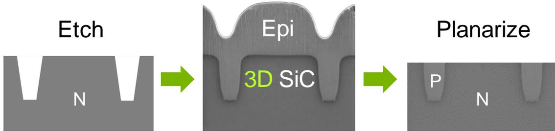
**Figure 2. Ascatron 3DSiC technology replaces ion implantation with epitaxial grown doping structures. This enables the design of high performance SiC power devices with stable high temperature operation. The superior material quality and design flexibility is also advantageous for realisation of high voltage devices with high current densities.**
