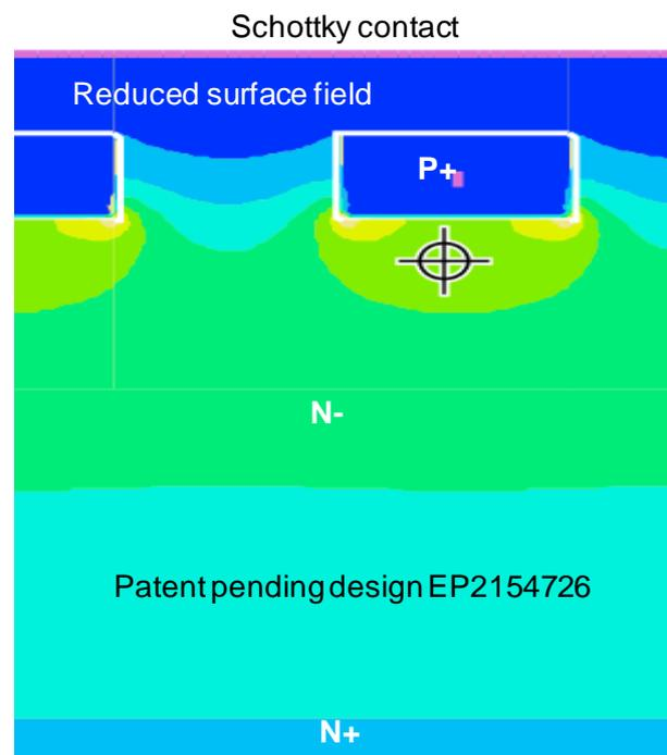
**Figure 1.** EPS diode design showing the simulated electrical field at blocking. The buried emitter grid reduces the leakage current, allowing operating temperature of 250°C.
